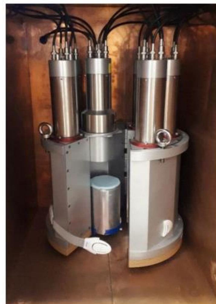
Figure 2. Unique gamma spectrometry system with an active anticoincidence shield.
